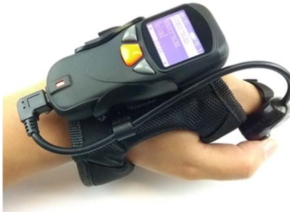
5. Connect trigger cable with pocket scanner and wear ring trigger unit. (you can use plastic hook to adjust the trigger cable.)
