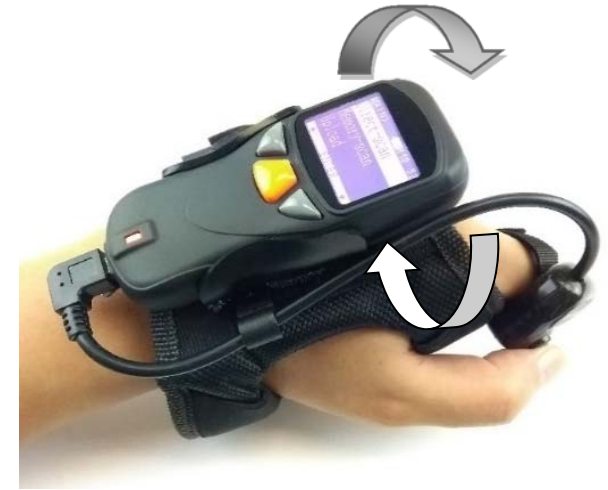
7. If you want to remove pocket scanner from Glove set, you can disassembled it as per above photo.
