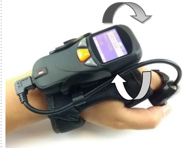
7. If you want to remove pocket scanner from Glove set, you can disassemble it as per above photo.
