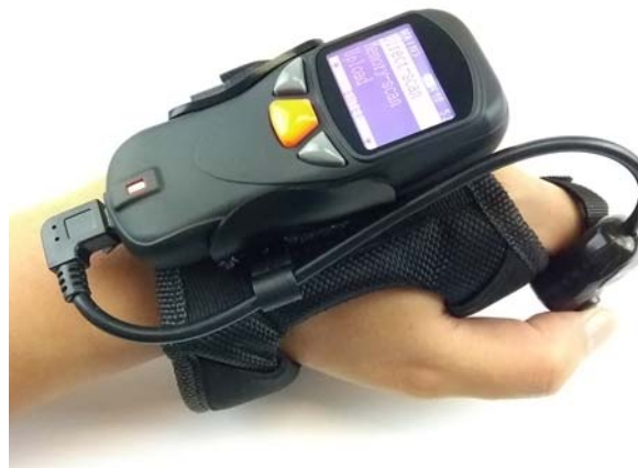
4. Put pocket scanner onto holder. (pay attention to assembling direction)
