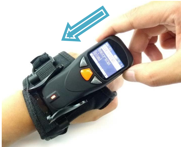
4. Put pocket scanner onto holder. (pay attention to assembling direction)
