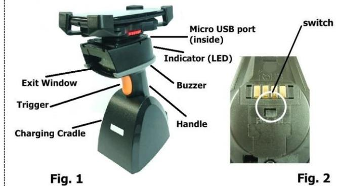
Scanner supports **BT communication mode** (for iOS and Android) and **wired OTG communication mode** (For Android OTG devices only/ For wired mode, you must shift the scanner's switch to "O"; followed by scanning the code of **Wired OTG communication mode** if you are shifting back from BT).
