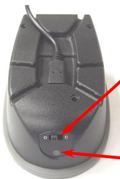
Before entering BT mode, you must switch to right "C" (Charging mode) first.
