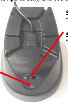
Switch to left: "O" (Operation mode) (data transmission)
