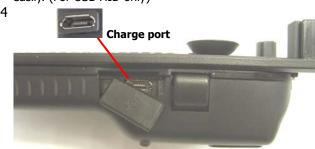
DC9277L is with Li-Ion battery inside. When in charging, please use the original power adaptor of OTG device (recommend). Through it, it charges both OTG device and DC9277L internal battery at the same time. When in low battery (Red LED flashing), please charge it immediately.
