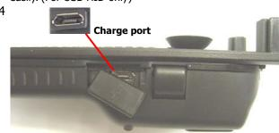
DC9277A is with Li-Ion battery inside. When in charging, please use the original power adaptor of OTG device (recommend). Through it, it charges both OTG device and DC9277A internal battery at the same time. When in low battery (Red LED flashing), please charge it immediately.
